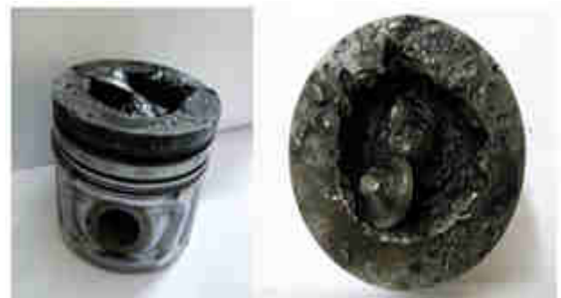
Fig.1: Piston with damaged crown portion.
